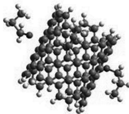
Fig. 7. Model of the adsorption interaction of nanotube (6, 6) and two molecules of n -propanol.
